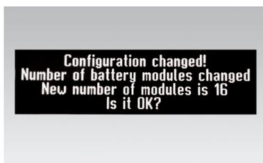
The display of the master APU HV1000-S now shows the number of detected battery modules (14 or 16). Confirm the number is correct by tapping twice. If there are deviations, shut down the TS HV 70 and check the BAT-COM wiring. If the fault continues to occur, contact service@tesvolt.com or the TESVOLT Service Line +49 (0) 3491 87 97 - 200.
