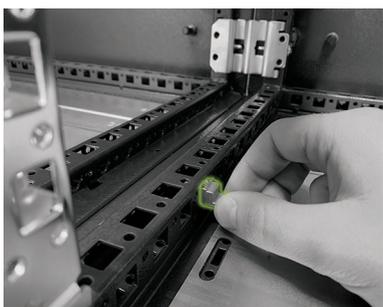
Fit the cabinet grounding connection set (K) to equalise the potential between the two halves of the cabinet. To do this, insert the speed nuts (K.5) from the side into the two middle cabinet profiles at the cabinet base. You are free to choose the position, but both speed nuts must be directly opposite each other.
