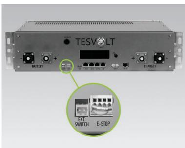
The four-pin plug for the e-stop connection on the APU HV1000-S must be plugged in for operation. The APU HV1000-S will remain inactive without this plug. Further information about the e-stop can be found in the section "6.3 E-stop contact" on page 30.
