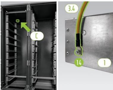
The APU HV1000-S must be grounded. Using the grounding cable (3.4), connect the APU HV1000-S to the central grounding point (C). To do this, place the grounding cable's M6 ring cable lug (3.4) onto the earthing bolt (14) (on the back of the APU HV1000-S) with a tightening torque of 6 Nm.
