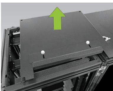
**Optional: lifting the cabinet covers for additional ventilation:** First of all, remove all the fastening screws, ring screws or combined brackets and then the two top cabinet covers.
