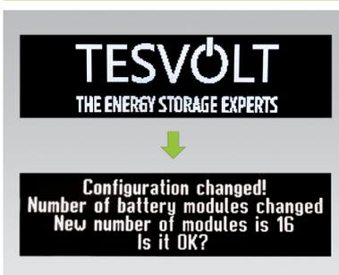
The number of battery modules detected (14 or 16) is shown on the display. Confirm the number is correct by tapping twice on the marking 16 beside the display. If the displayed number of modules differs from the number actually present, shut down the unit and check the BAT-COM wiring. If the fault continues to occur regardless, please contact the TESVOLT Service Line +49 (0) 3491 8797-200 or email to service@tesvolt.com.
