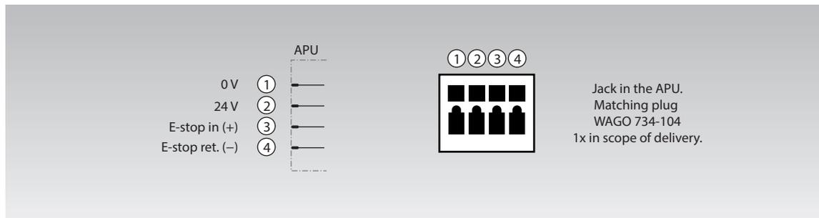
Figure 6.2 Assignment of the e-stop connection jack 4
