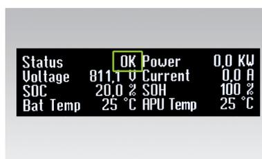
Once the precharging has completed successfully, the on/off switches "SWITCH" 17 on all APU HV1000-Ss in the master/slave configuration are continuously illuminated. "OK" appears as the status on the display of the APU HV1000-S. All the TS HV 70 units are now ready for operation.
