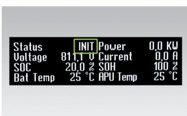
The TS HV70 switches to "INIT" mode and the on/off "SWITCH" 17 starts to flash.
