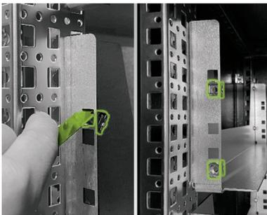
Fit the cage nuts (J) for affixing the APU HV1000-S (1) in the slide rails using the auxiliary tool (J1). The APU HV1000-S uses the top slide rails in the left half of the cabinet. Distribute the cage nuts from bottom to top. Start at the bottom edge of the slide rails of the APU HV1000-S. Use the first opening and fit the first two cage nuts on both sides. Now, fit the remaining two cage nuts in the second opening in both slide rails from the top.
