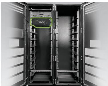
Insert the first battery module into the slide rails below the APU HV1000-S. Affix it to the pre-fitted cage nuts using four M6 x 16 pan head screws (I) (cross-head) incl. plastic washers (I.I). Now fit the remaining modules in the left half of the cabinet. If 16 battery modules are being used, the bottom position is occupied as well.
