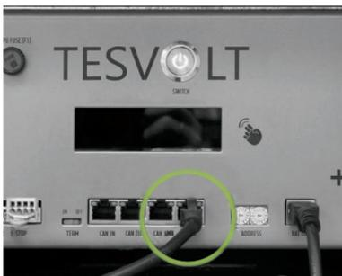
Establish the **LAN connection** (9) for the APU HV1000-S using the patch cable (7.4) with one of the two supplied TESVOLT switches (8) and with the jack labelled "LAN". This switch is connected to the "LAN 2" jack of the SMA Inverter Manager (10) and will be referred to as the "LAN 2 switch" from now on. The SMA STPS 60 is also connected to it (see section "7 Connection to the battery inverter" on page 32 et seq.).
