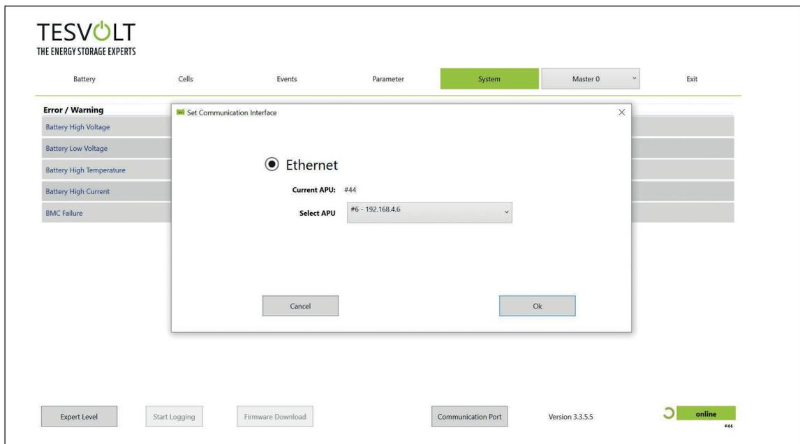
Figure 12.1 Screen for setting the network configuration
