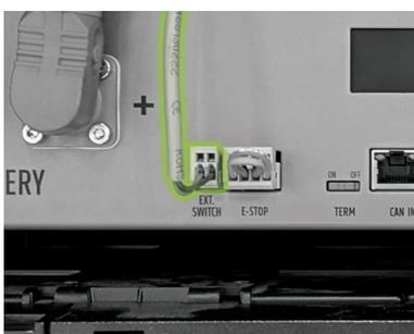
Insert the plug of the connection cable (E) into the "EXT. SWITCH" connection (3) on the APU HV1000-S.
