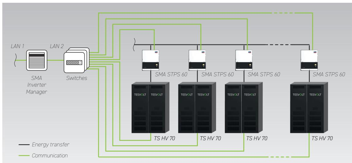
The charging and discharging power can be increased by increasing the number of SMA STPS 60 units. Up to 20 SMA STPS 60 units can be operated on one SMA Inverter Manager.
