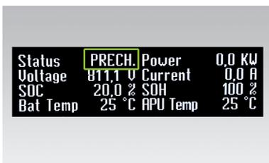
Start the commissioning process of the battery inverter with the SMA LCS Tool. The software and a manual can both be found on the TESVOLT USB-Stick 16. Once the commissioning process has been successfully completed, the battery storage system switches to pre-charge mode "PRECH".
