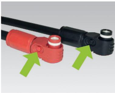
When installing the DC wiring, please note the following: **the plugs must audibly click into place.** The plugs can be unlocked by pressing the pushbutton on the side of the plug (see markings in the illustration).
