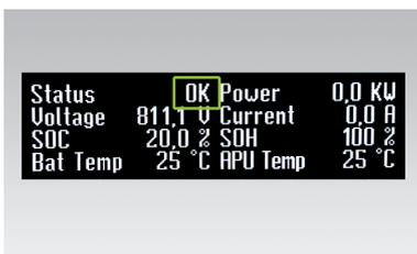
After precharge mode, the on/off "SWITCH" 17 remains lit. "OK" appears as the status on the display of the APU HV1000-S. The TS HV70 is now ready for operation.
