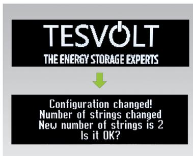
Unlike the slave APUs, the master initially requests the number of "strings". The number of strings corresponds to the number of storage systems in the master/slave configuration (e.g. master + slave 1 = 2 strings). Confirm the number is correct by tapping twice next to the display. If there are deviations, check the CAN OUT → CAN IN wiring, the termination and the addressing. If the fault continues to occur, contact the TESVOLT Service Line +49 (0) 3491 87 97 - 200 or service@tesvolt.com.
