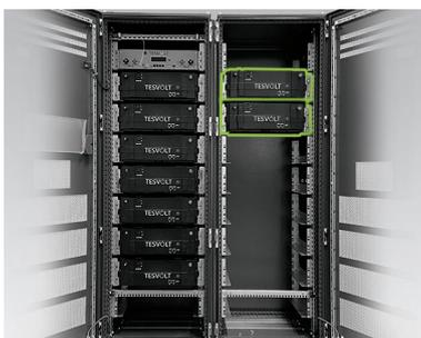
Once the left half of the cabinet has been filled, install the battery modules on the right side. Start at the level of the top left module (the position at a level with the APU HV1000-S remains unoccupied). Affix the module to the pre-fitted cage nuts (J) with four M6 x 16 pan head screws (I) incl. washers (I.I). Then, place the next module below the one that has already been installed and fasten it as described. Continue until all the modules have been installed.
