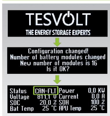
The number of battery modules detected (14 or 16) is shown on the slave storage system's display. Confirm the number is correct by tapping twice on the marking 16 next to the display. If the displayed number of modules differs from the number actually present, shut down the TS HV70 and check the BAT-COM wiring.
