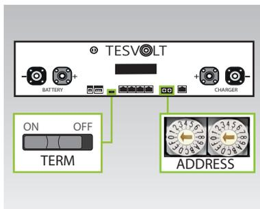
Check and, if necessary, correct the settings for termination and addressing the TS HV 70 ("TERM" 5 and "ADDRESS" 10) on the APU HV1000-S.
