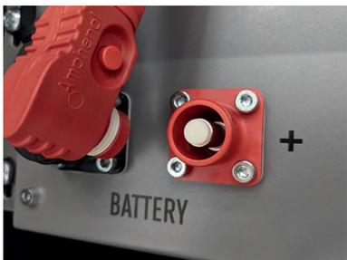
To ensure a long battery life, the storage temperature should be kept in a range between  $-20^{\circ}\text{C}$  and  $50^{\circ}\text{C}$  and the cells should be cycled at least every six months. To minimise self-discharge during longer storage periods, the DC connection cables should be removed from the "BATTERY" connections ①/② of the APU HV1000-S. This interrupts the power supply of the 24 V power supply installed in the APU HV1000-S and prevents discharge of the battery.
