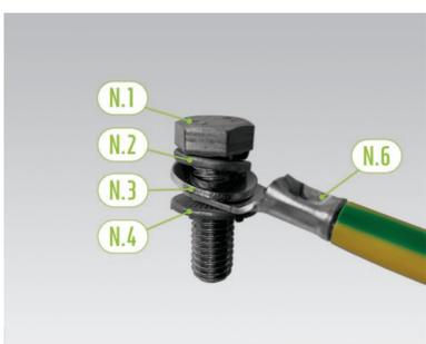
Now prepare the grounding cable (M.6) for installation. To do this, put an M8 spring washer (M.2), an M8 washer (M.3), the grounding cable's cable eyelet (M.6) and finally the M8 contact washer (M.4) onto the M8 screw (M.1). Ensure that the teeth of the M8 contact washer (M.4) are pointing downwards, towards the end of the screw.
