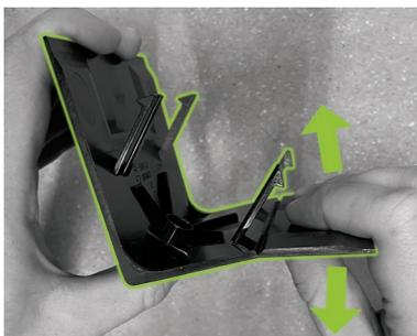
Prepare a right base corner cover plate (G) (with the logo on the left leg) for fitting on the cabinet base. To do this, break the cover plate in half at the notch on the right leg. The narrow piece can be disposed of. Now use the two hooks of the connector for the base corner cover plate (G.2) to attach it to the shortened cover plate's short leg.
