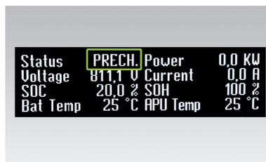
Start the commissioning process of the SMA STPS 60 with the SMA LCS Tool. The software and a manual can both be found on the TESVOLT USB-Stick 16. Once the commissioning process has been successfully completed, all the TS HV 70 units switch to precharge mode "PRECH".
