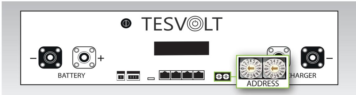
Set the address selector on the APU HV1000-S to match the configuration and data in the table below.
