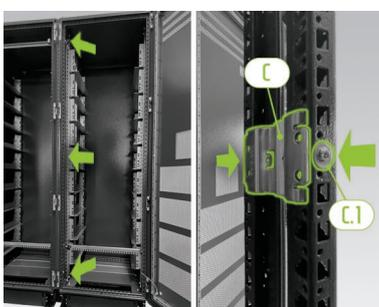
First of all, on the front of the cabinet attach three baying connectors (H) to the middle, vertical cabinet profiles inside the cabinet at the top, middle and bottom. The baying connectors are affixed to the frame profiles with two setscrews (H.1) on each side from the right and left.
